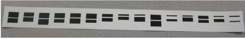
Fig. 2. Marker design with projective invariant pattern properties
