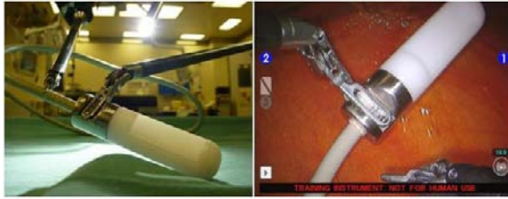
Fig. 2. The pick-up IAUS transducer is grasped and manipulated by the Pro-Grasp tool of the da Vinci Surgical System
